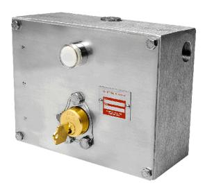
The Type SKRU consists of an interlock, a solenoid, and an auxiliary switch. The solenoid is designed to permit removal of the interlock key in response to an external electric signal. The auxiliary switch is a quick-make, quick-break device, which operates when the interlock key is rotated. Normally, the key is trapped in the SKRU and the solenoid is de-energized. To release the key, a signal must be sent to the solenoid from an external source.
